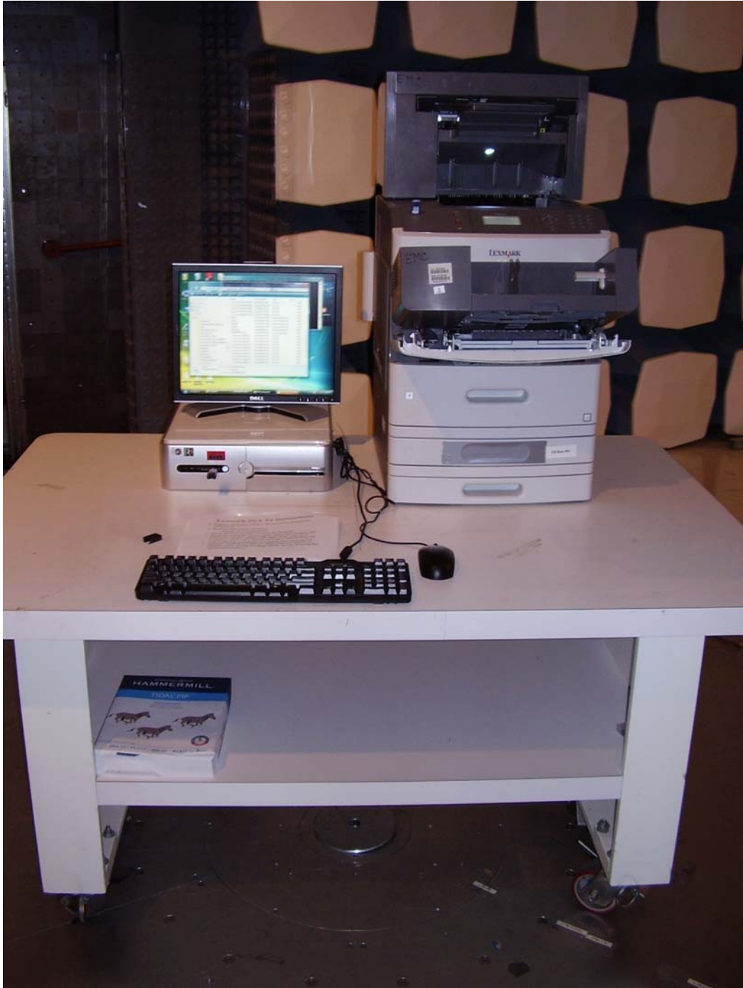
Test configuration for transmitter radiated spurious emissions (front view).
