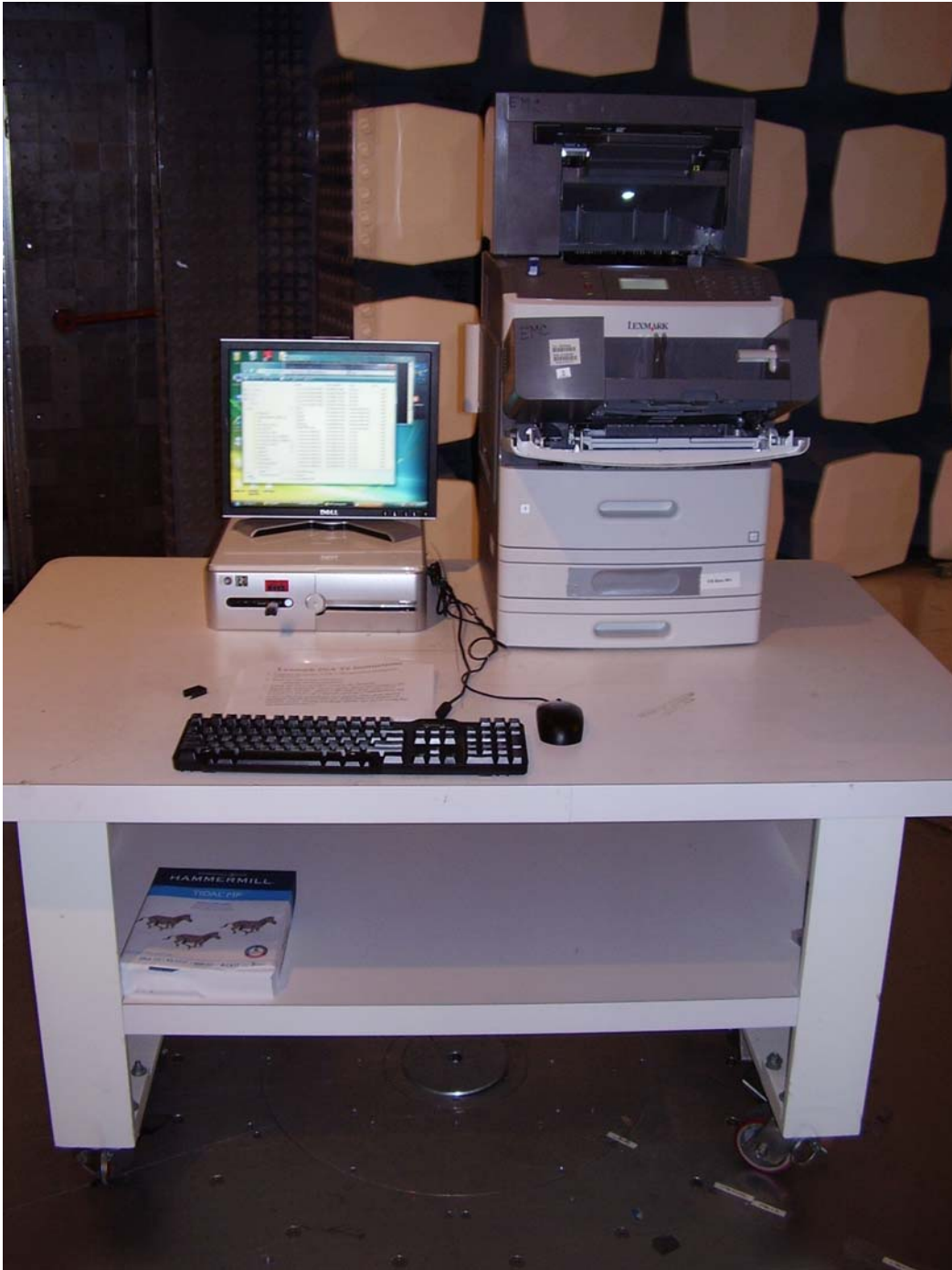
Figure 44. Test configuration for transmitter spurious emissions (front view).
