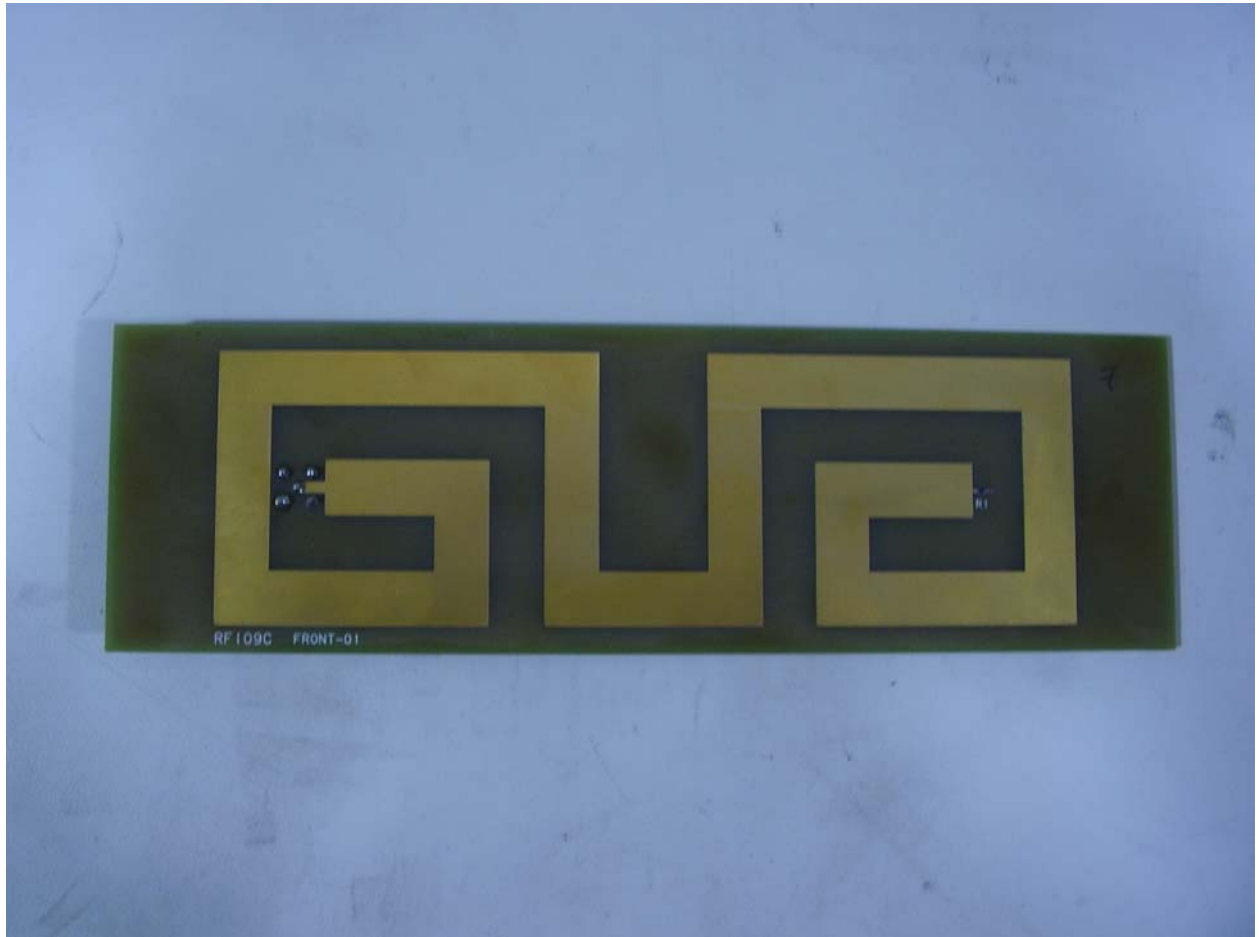
Front view of antenna.
