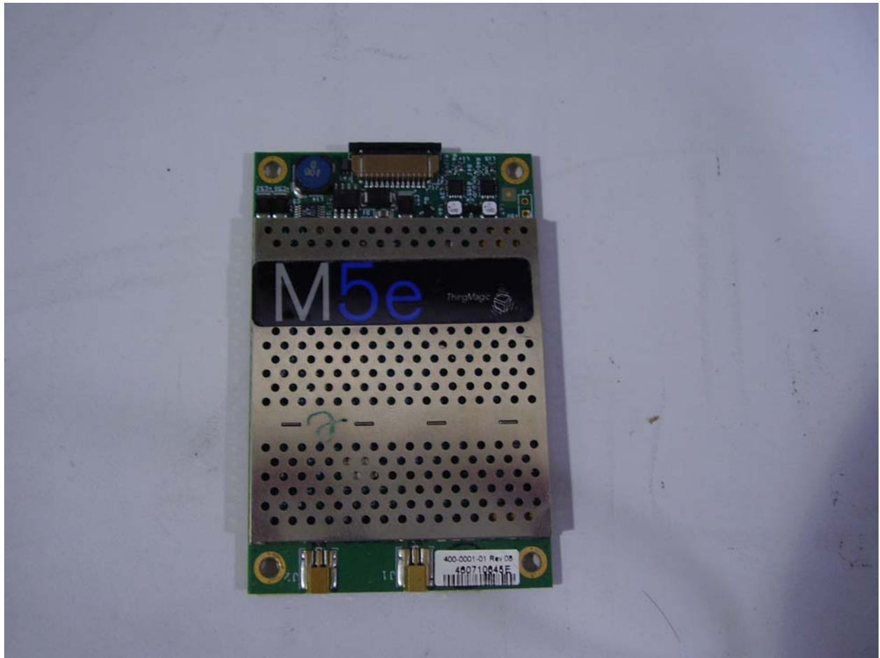
Front view of radio card.
