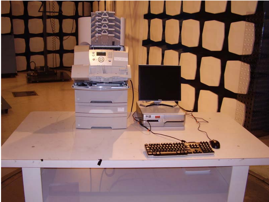
Figure 44. Test configuration for transmitter spurious emissions (front view).
