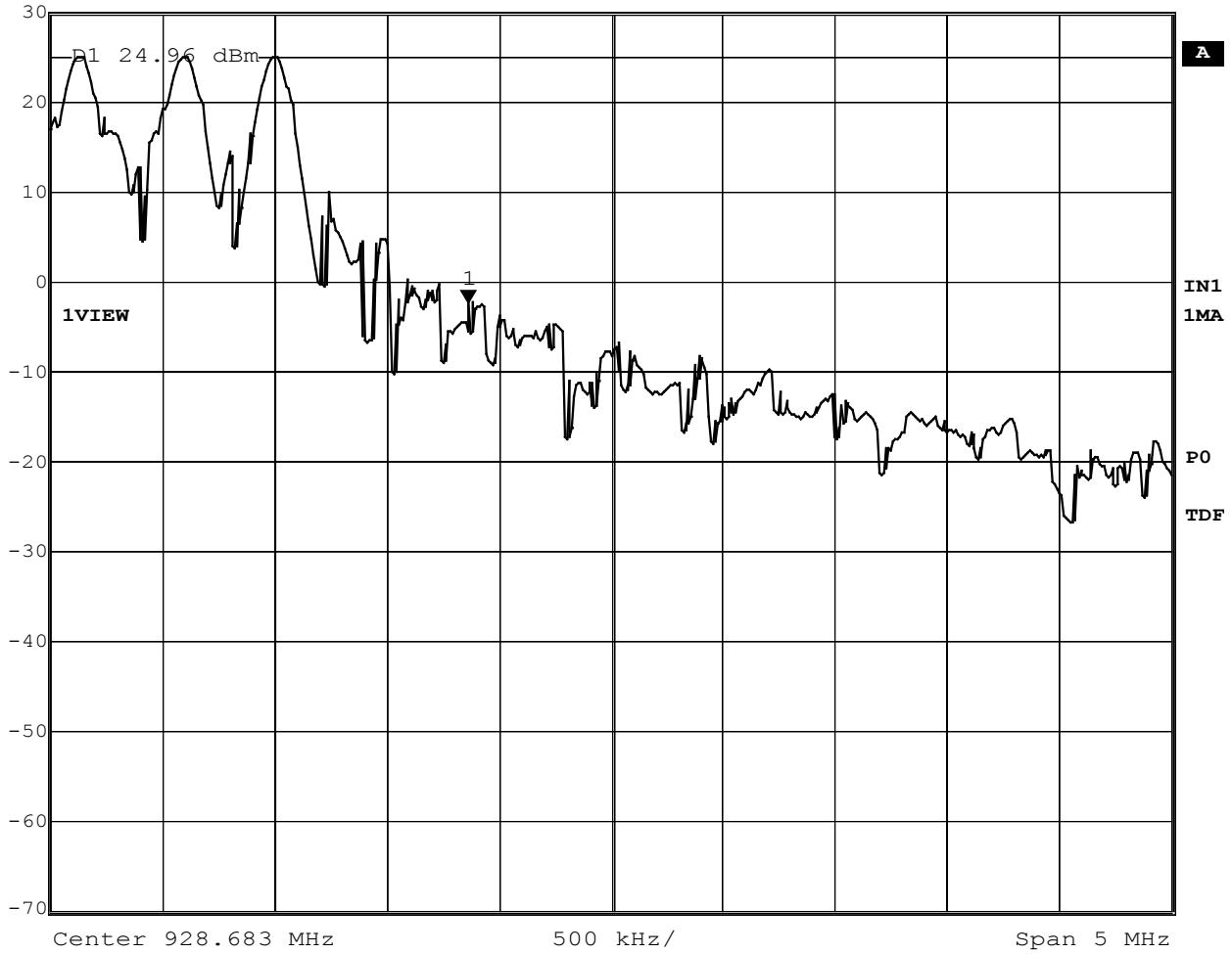
Figure 43. Band edge compliance; EPC Gen2 mode; Channel 53, hopping enabled.
