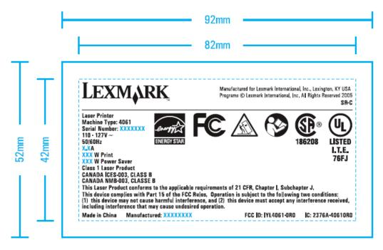
Label is made of a polyester film material with laser printable top coating.
