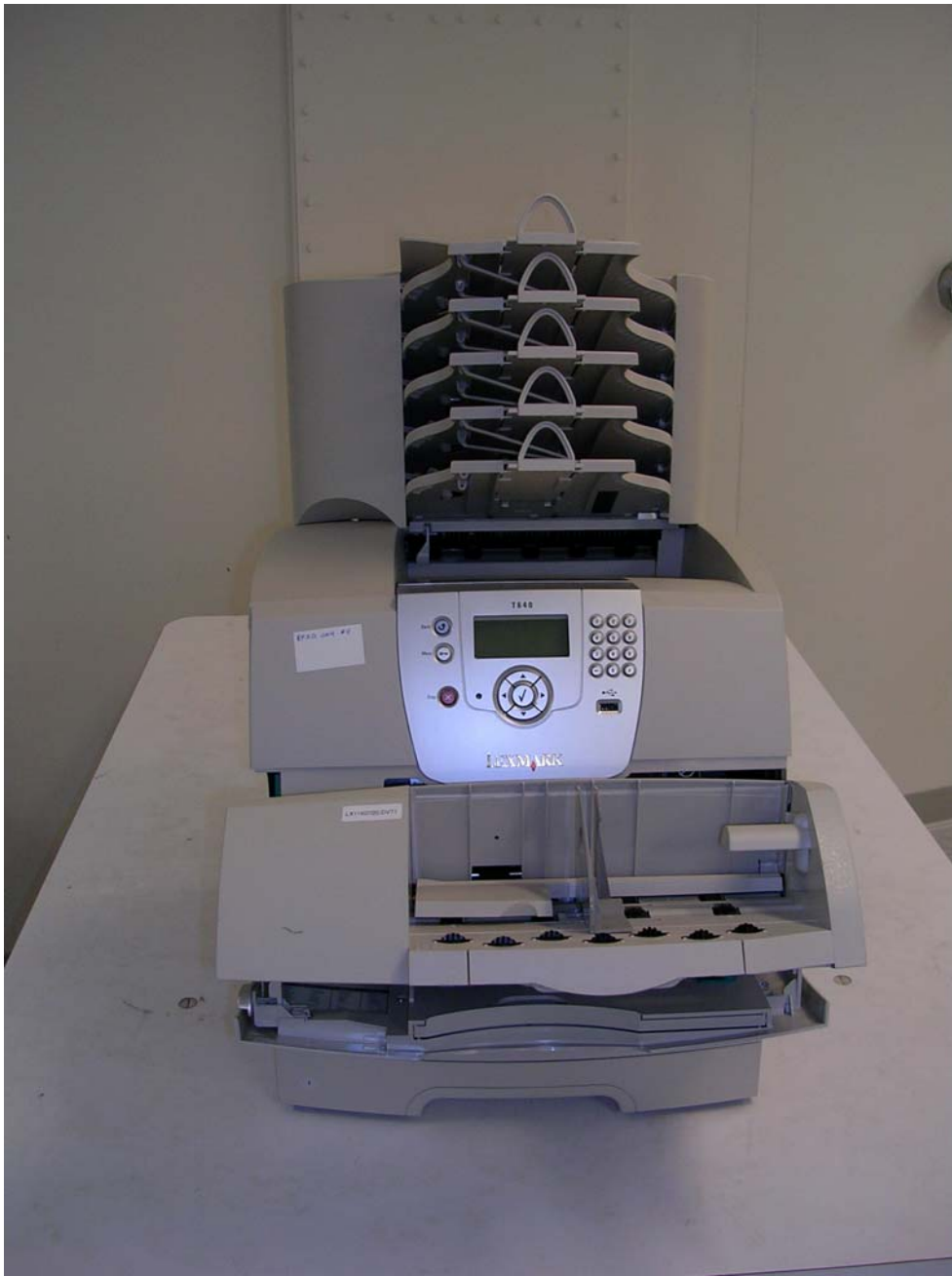
Front of printer. Shown with optional top output bin, envelope feeder and paper drawer.
