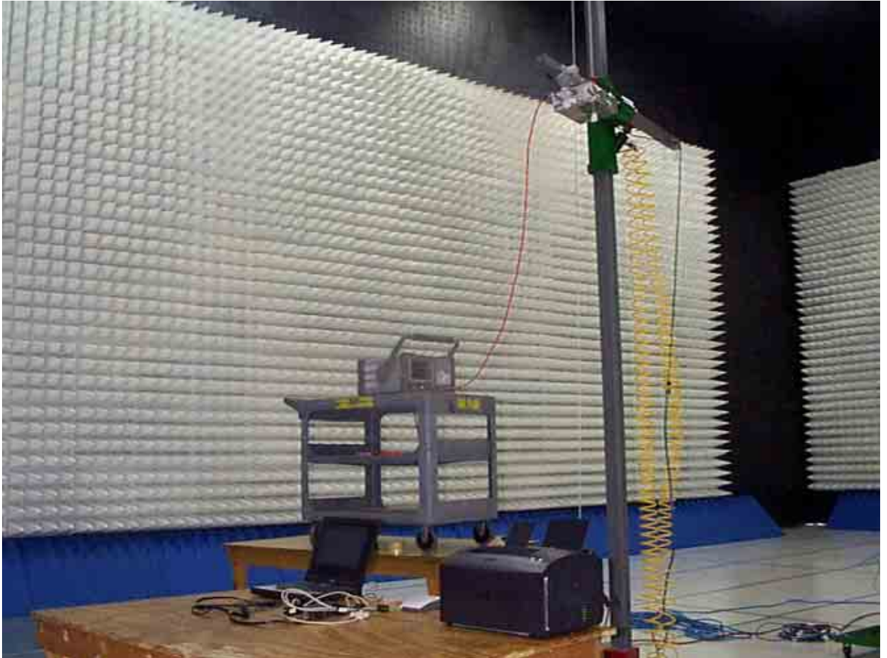
Figure 3: Radiated Testing to 26GHz
