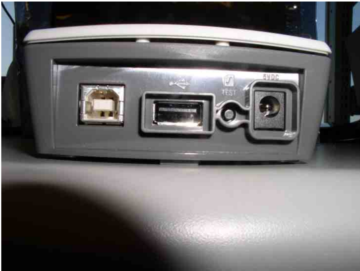
Rear View (Showing Cable Connections)
