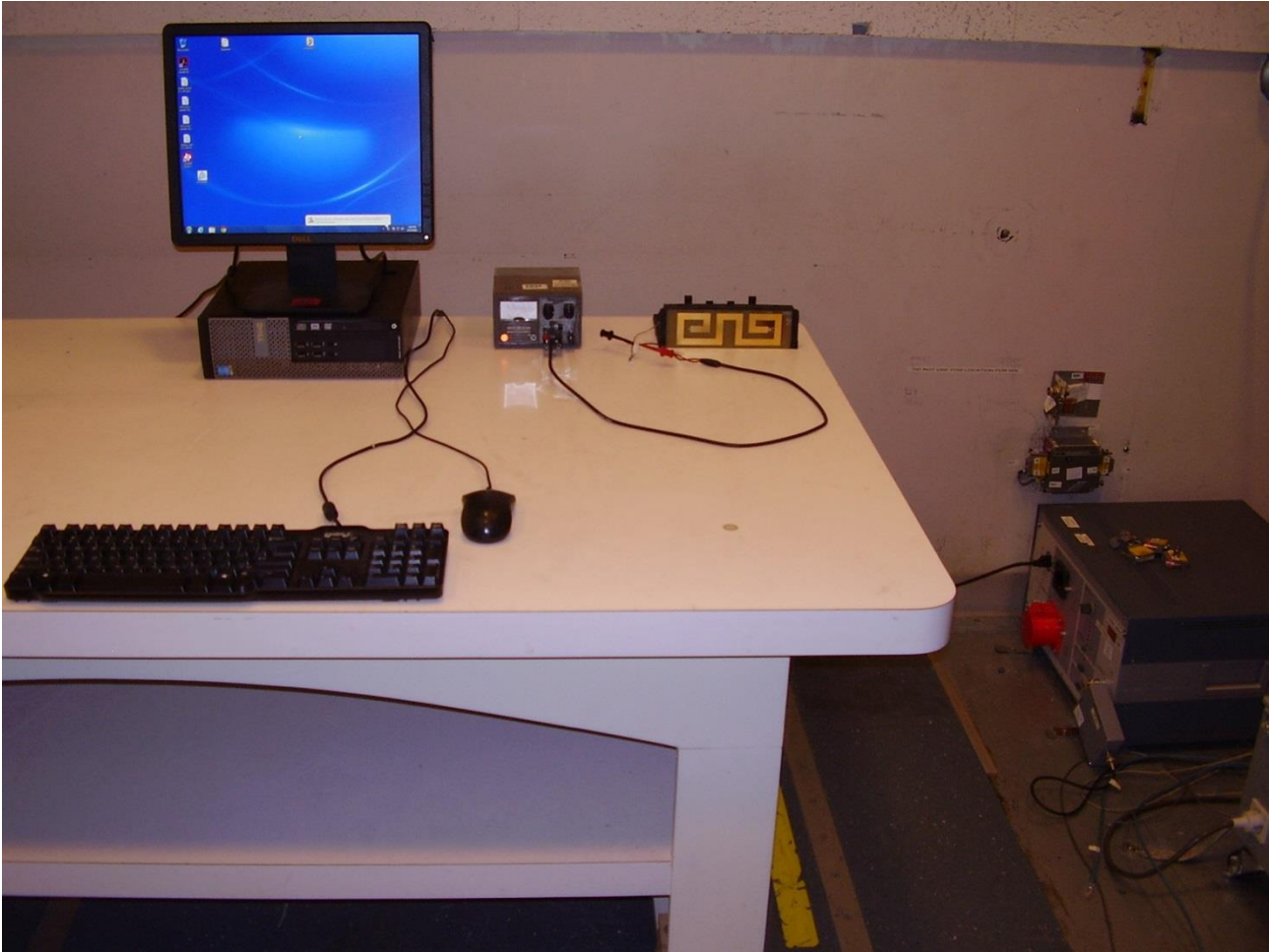
Figure 41. Test setup for AC conducted emissions.
