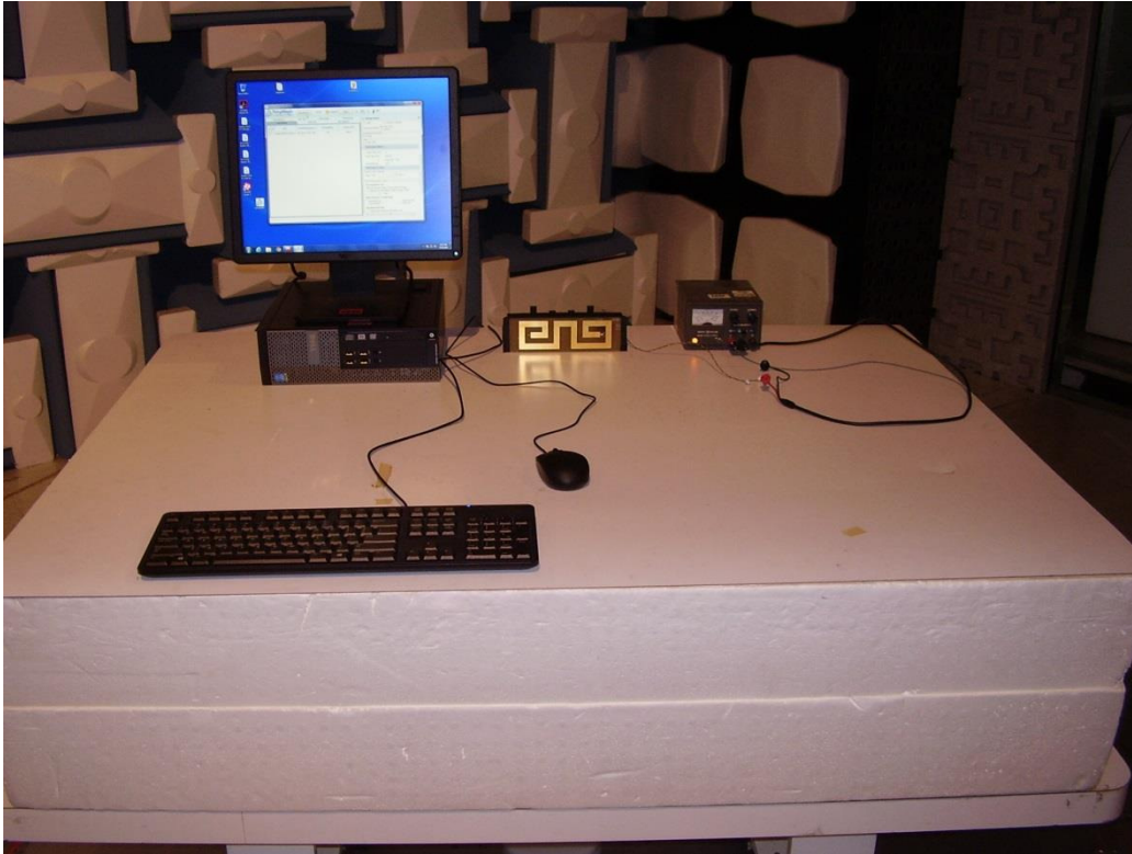
Figure 31. Test setup for radiated spurious emissions 30 MHz – 1000 MHz; front view.
