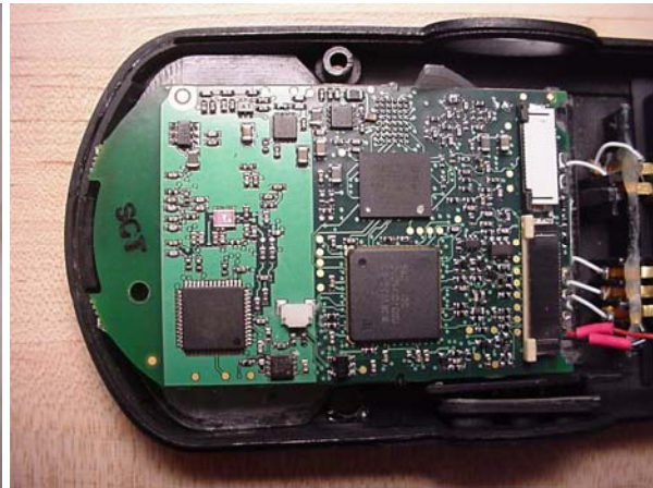
RNP2400 RF Generation Board – Side B
