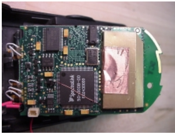
RNP2400 RF Generation Board – Side A
