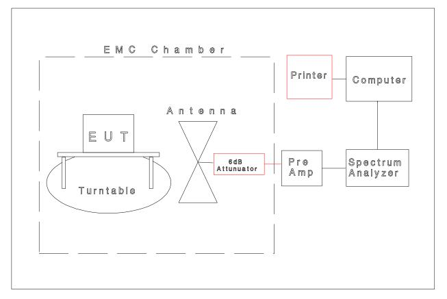
Radiated Emissions Test
