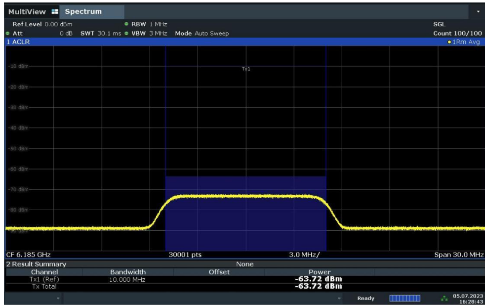
AWGN Signal Level 802.11ax HE160 6185 (middle, at Antenna Port)
