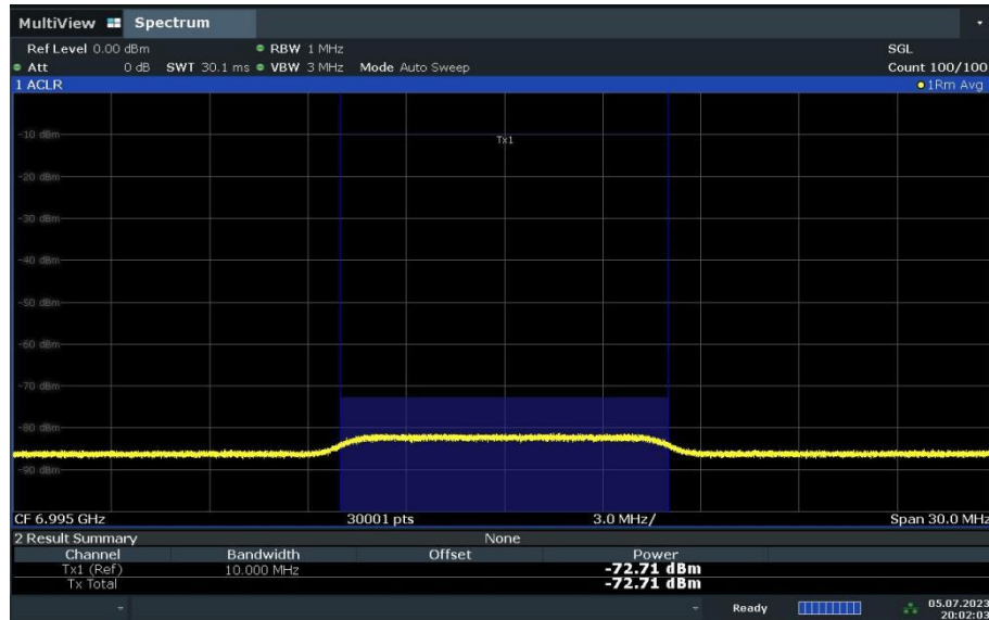
AWGN Signal Level 802.11ax HE20 6995MHz (at Antenna Port)
