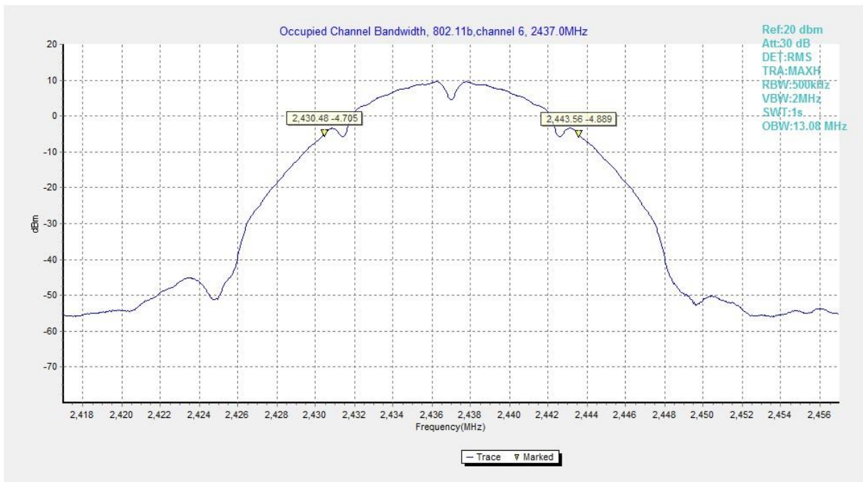
Fig.2 99% Occupied Bandwidth (802.11b, CH 6)
