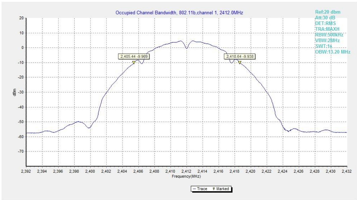
Fig.1 99% Occupied Bandwidth (802.11b, CH 1)
