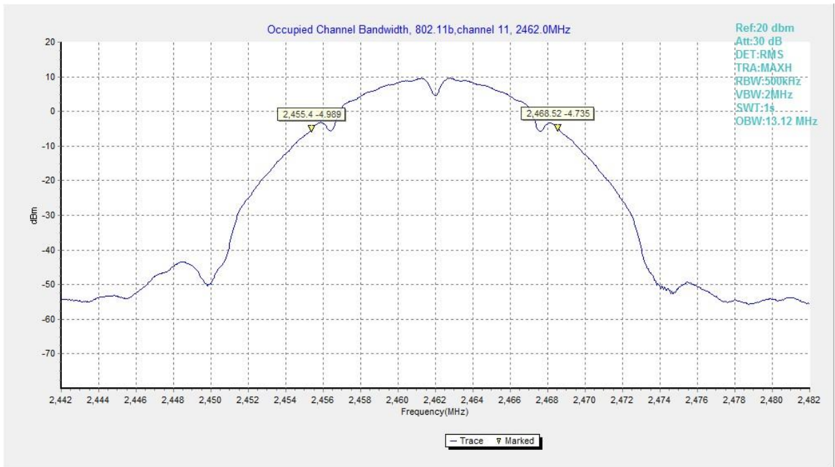
Fig.3 99% Occupied Bandwidth (802.11b, CH 11)
