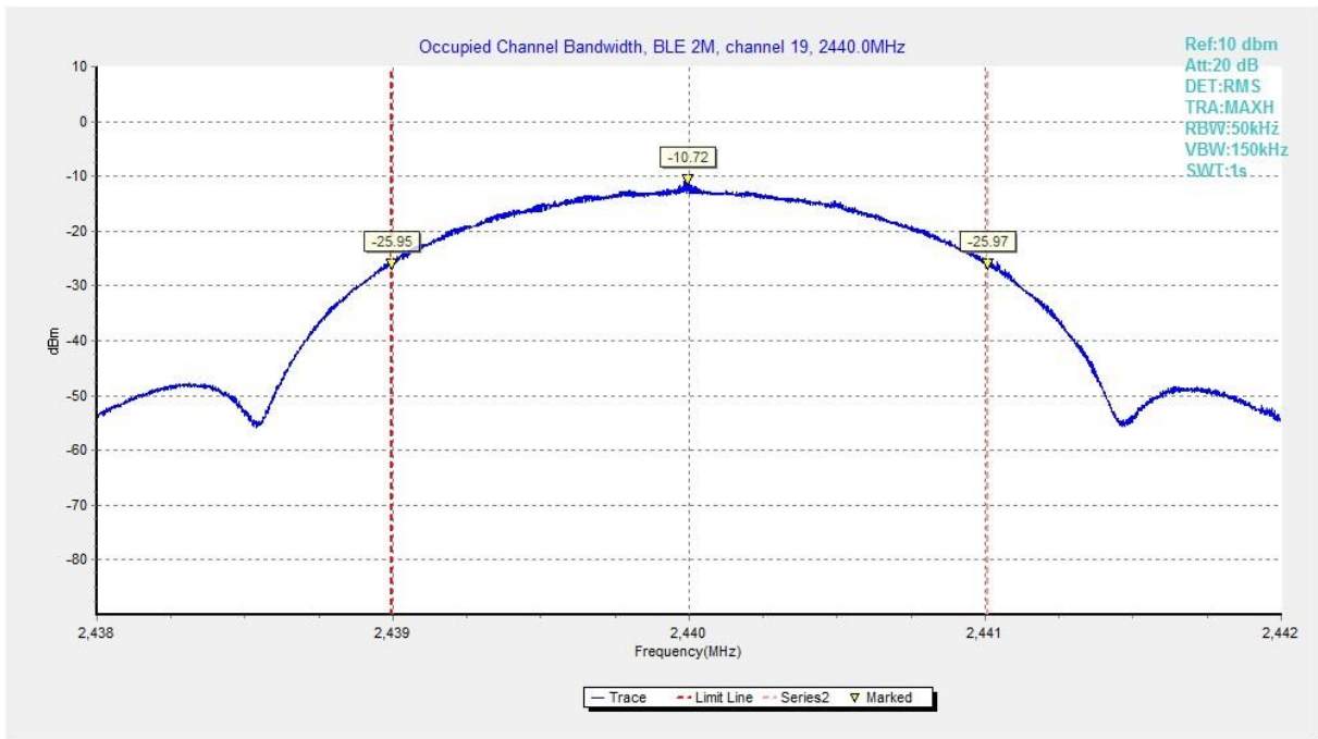
Fig.2 99% Occupied Bandwidth (Ch 19), LE 2M
