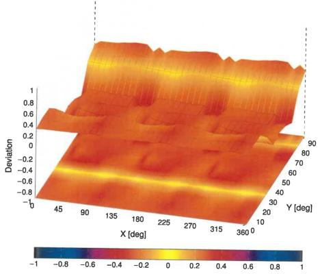
Probe isotropy for E<sub>tot</sub>: probe rotated  $\phi$  = 0° to 360°, tilted from field propagation direction  $\vec{k}$ Parallel to the field propagation ( $\psi$  = 0° - 90°) at 30 GHz: deviation within ±0.31 dB Parallel to the field propagation ( $\psi$  = 0° - 90°) at 60 GHz: deviation within ±0.36 dB
