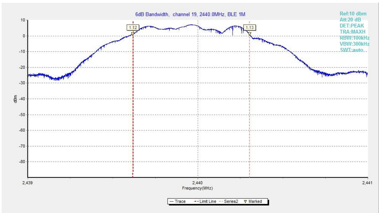
Fig.3 6dB Bandwidth (Ch 19), LE 1M
