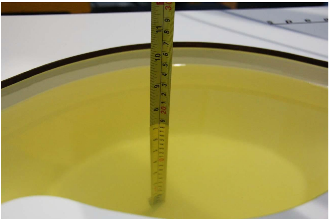
Picture 7-10: Liquid depth in the Flat Phantom(2450MHz)
