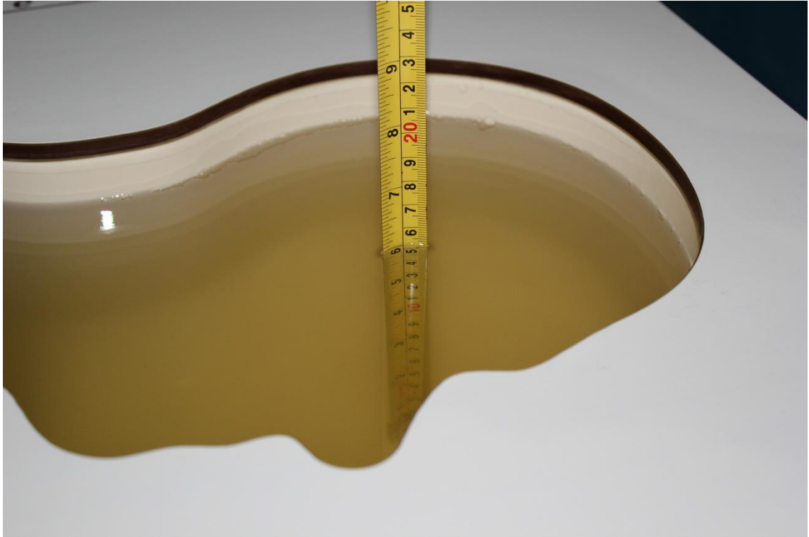
Picture 7-11: Liquid depth in the Head Phantom(2550MHz)
