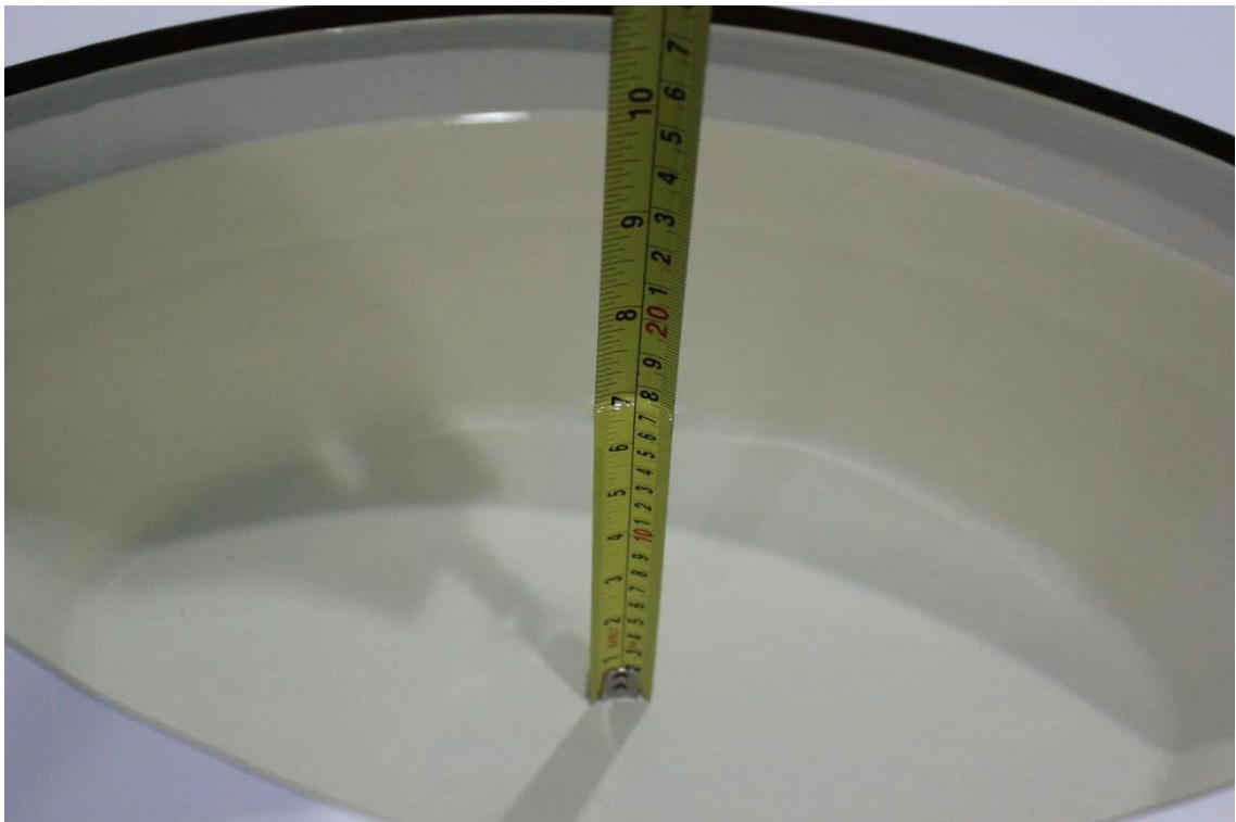
Picture 7-4: Liquid depth in the Flat Phantom (5GHz)
