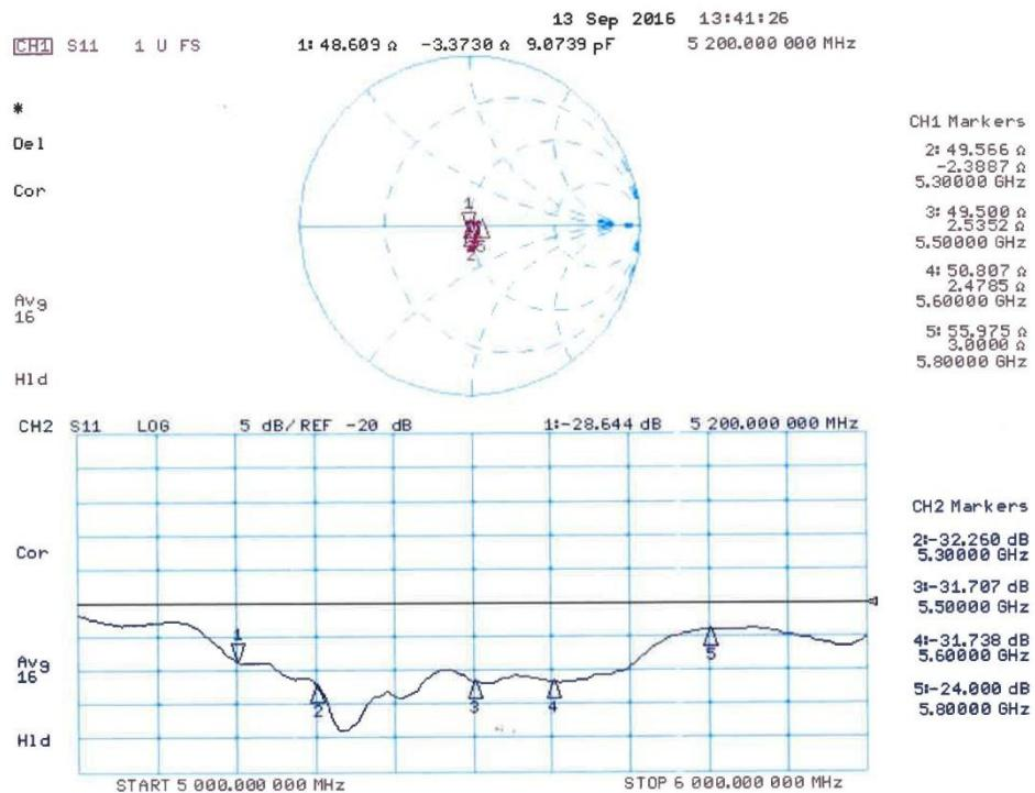
**ANNEX J Extended Calibration SAR Dipole**
