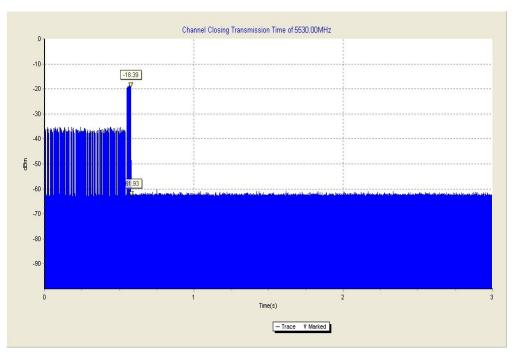
The closing transmission time is as the figure, and the result is 6ms.
