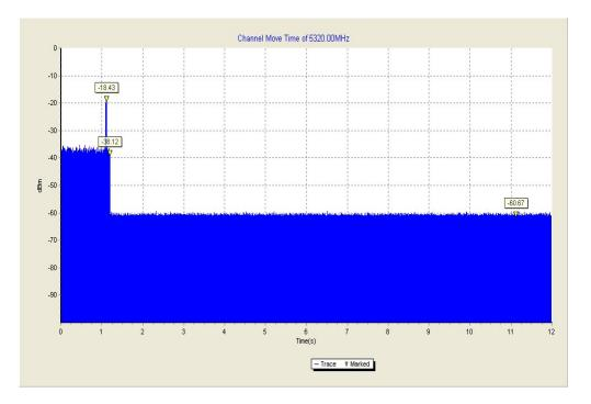
The channel move time is as the figure. It shows the time of the radar and the client pulses. The figure shows that the client stops transmission within 10 seconds, and no transmissions occur after 10 seconds later of the radar burst signal.
