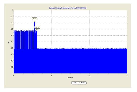
The closing transmission time is as the figure, and the result is 63ms.
