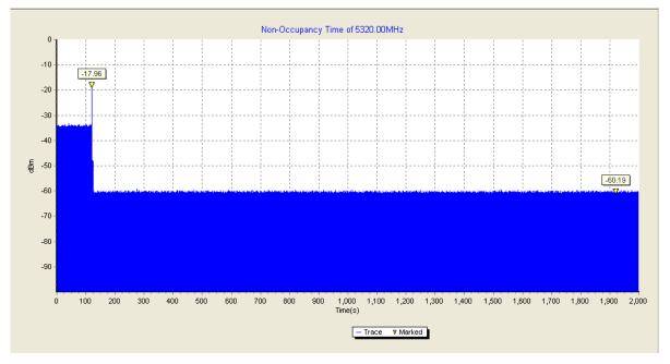
The figure above shows that the client does not transmit any emission within 1800 seconds after getting the order of "stop transmits" from the DFS master (access point).
