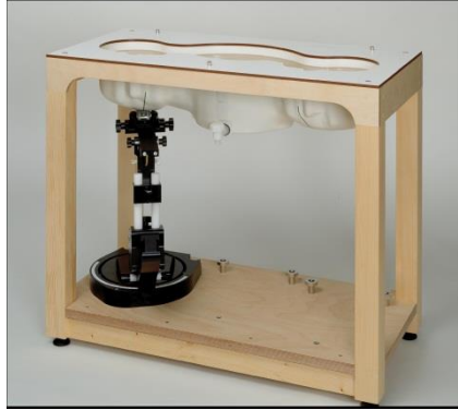
Picture C.8: SAM Twin Phantom
