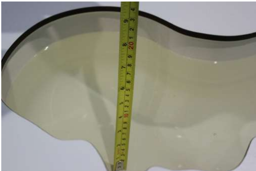
Picture 7-2: Liquid depth in the Head Phantom(5GHz)
