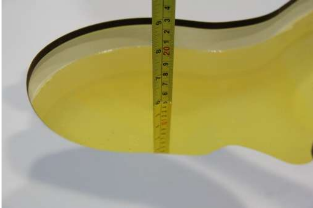
Picture 7-1: Liquid depth in the Head Phantom(2450MHz)
