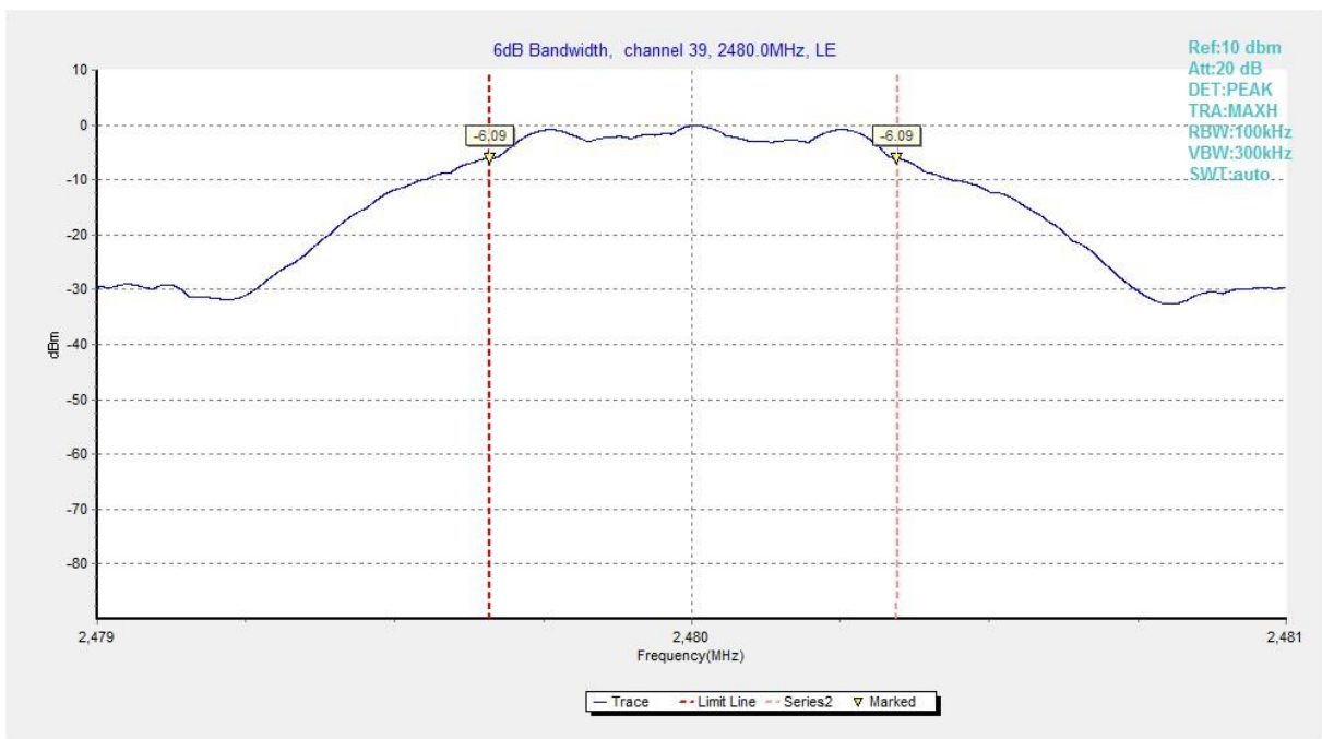
Fig.6 6dB Bandwidth (Ch 39)
