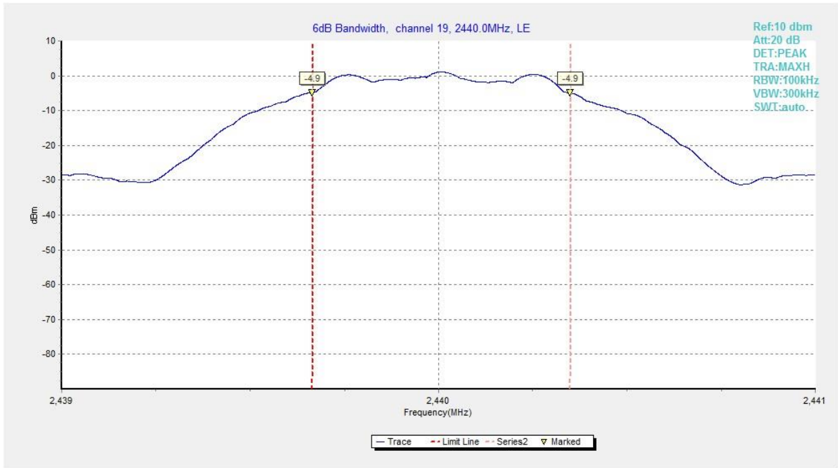
Fig.5 6dB Bandwidth (Ch 19)
