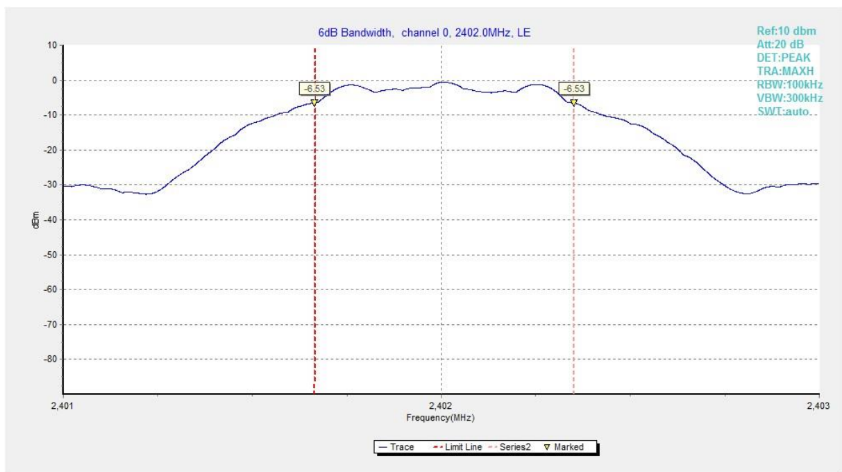
Fig.4 6dB Bandwidth (Ch 0)
