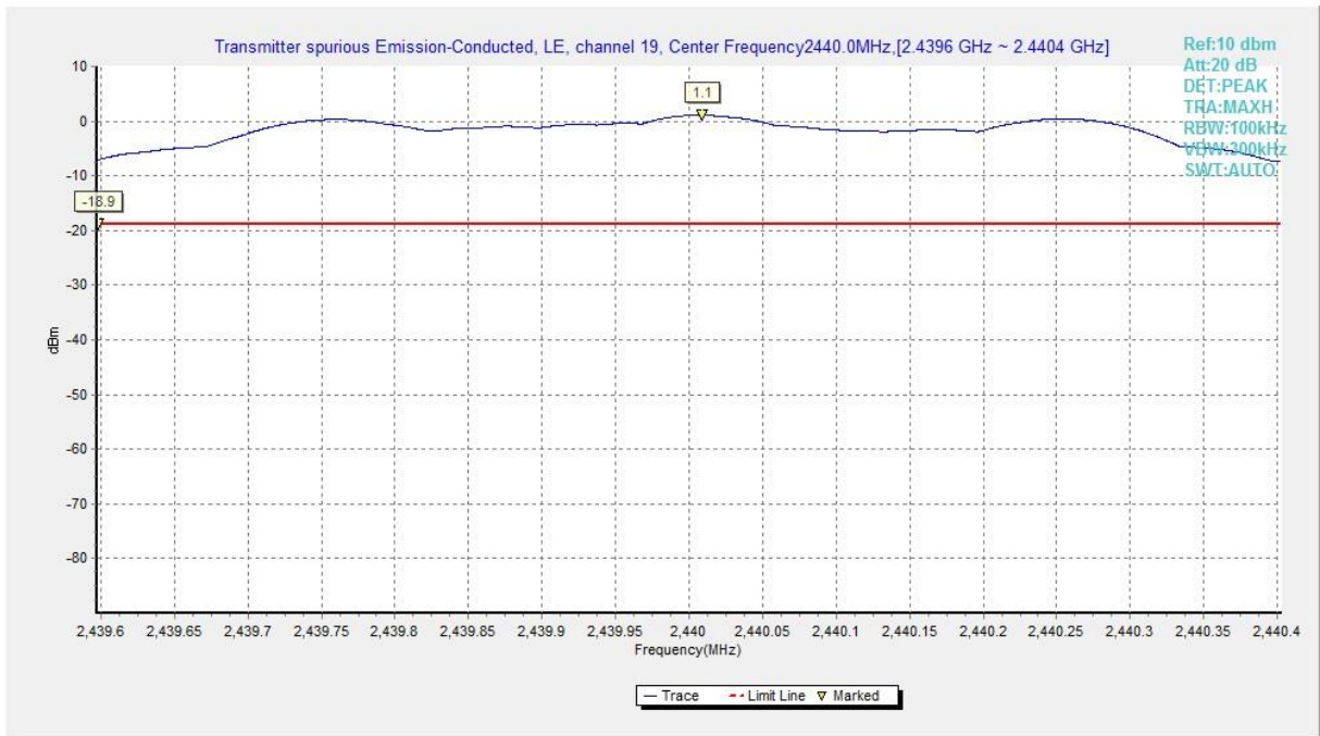
Fig.12 Conducted Spurious Emission (Ch19, Center Frequency)
