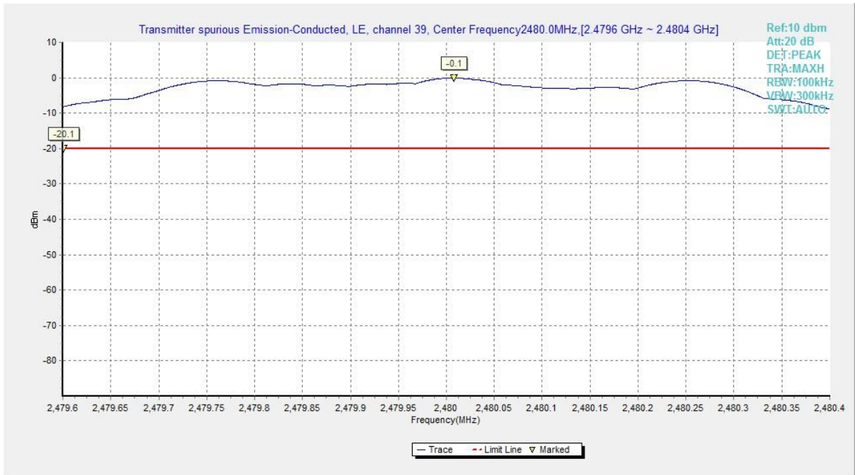
Fig.15 Conducted Spurious Emission (Ch39, Center Frequency)
