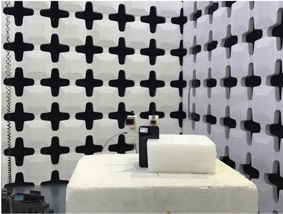
13. Radiated Emissions (Part 15C&Part 15E, 26.5GHz -40GHz)
