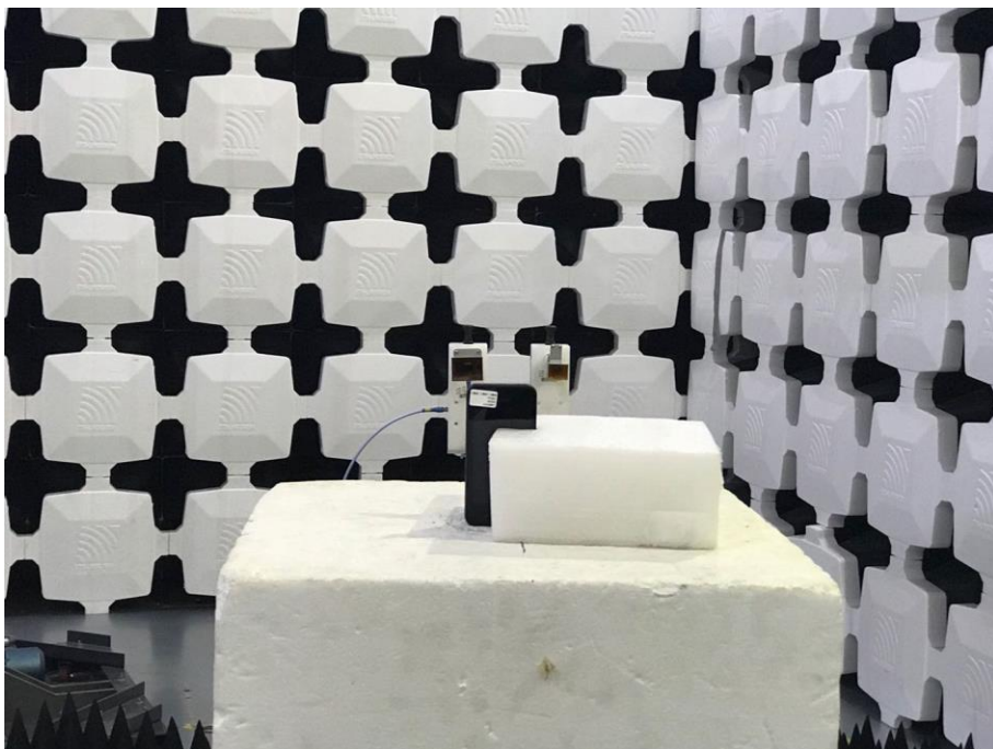
12. Radiated Emissions (Part 15C&Part 15E, 18GHz -26.5GHz)
