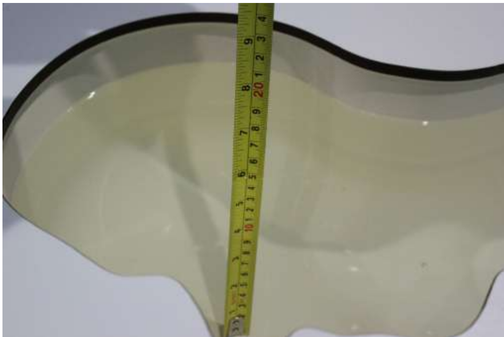
Picture 7-2: Liquid depth in the Head Phantom(5GHz)
