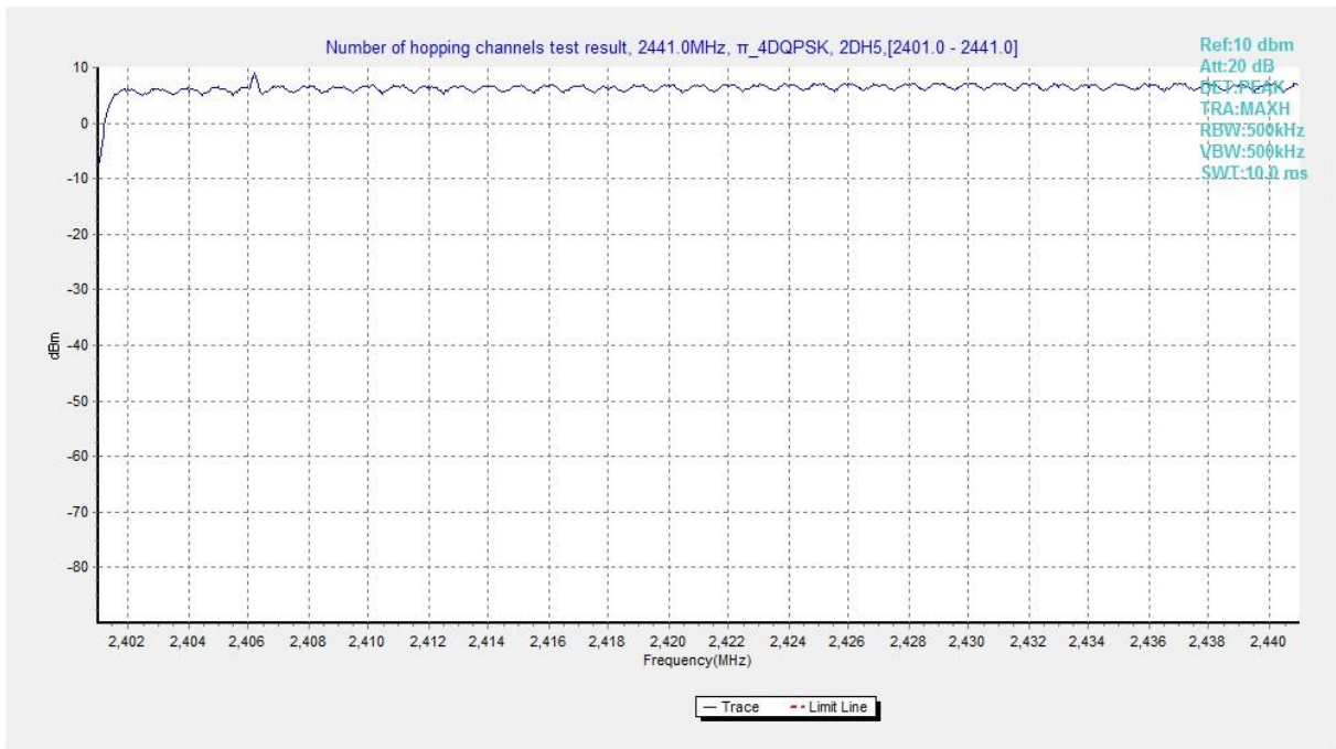
Fig. 77 Hopping channel ch0~39 ( \pi/4 DQPSK, Ch39)
