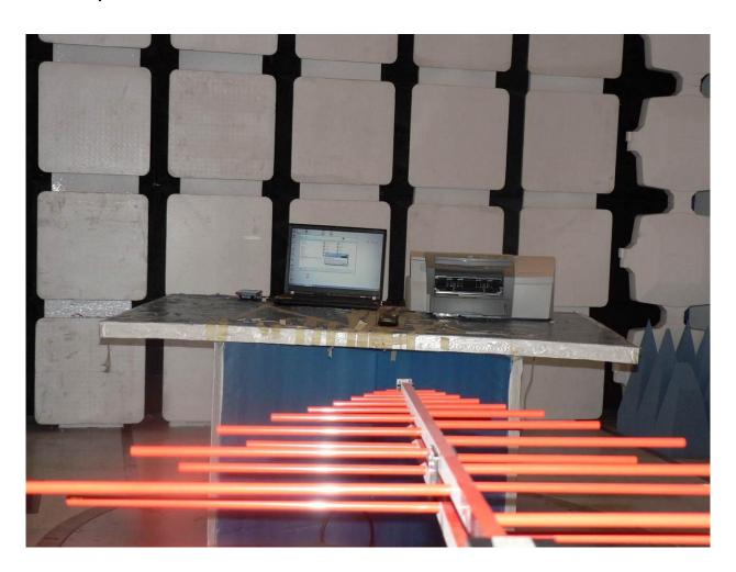
Test Setup – Radiated Emissions #2
