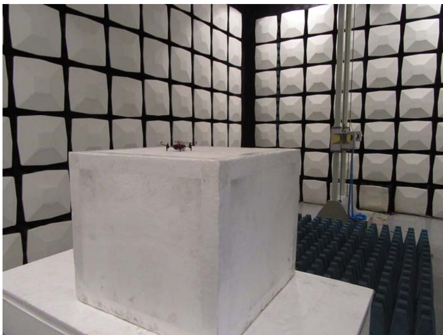
Radiated Emission View (Above 1GHz)
