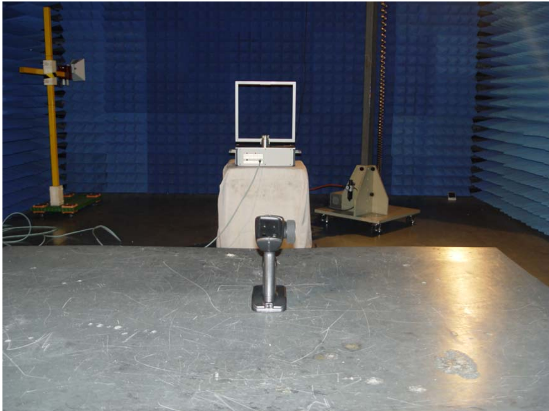
Radiated emissions test < 30MHz
