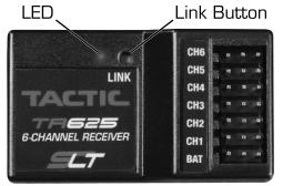
CH6 Auxiliary (Flaps) CH5 Auxiliary (Landing Gear)
