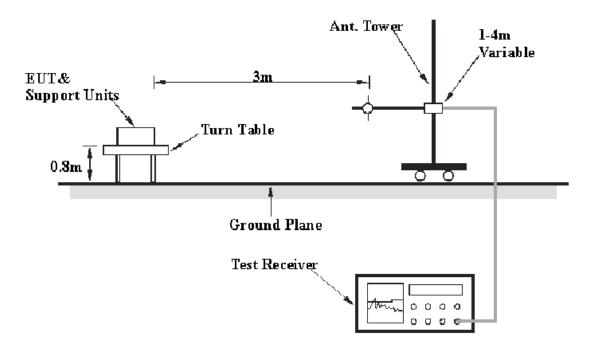
The radiated emission tests were performed in the 3 meters, using the setup accordance with the ANSI C63.4-2009. The specification used was the FCC 15.209, and FCC 15.247 limits.
