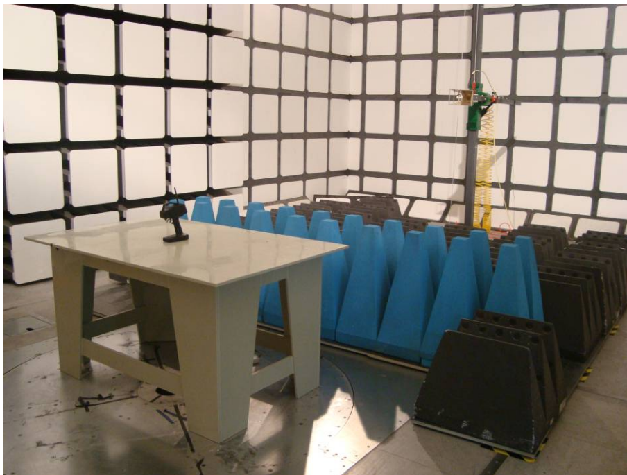
Above 1 GHz: Radiated Emissions - Rear View
