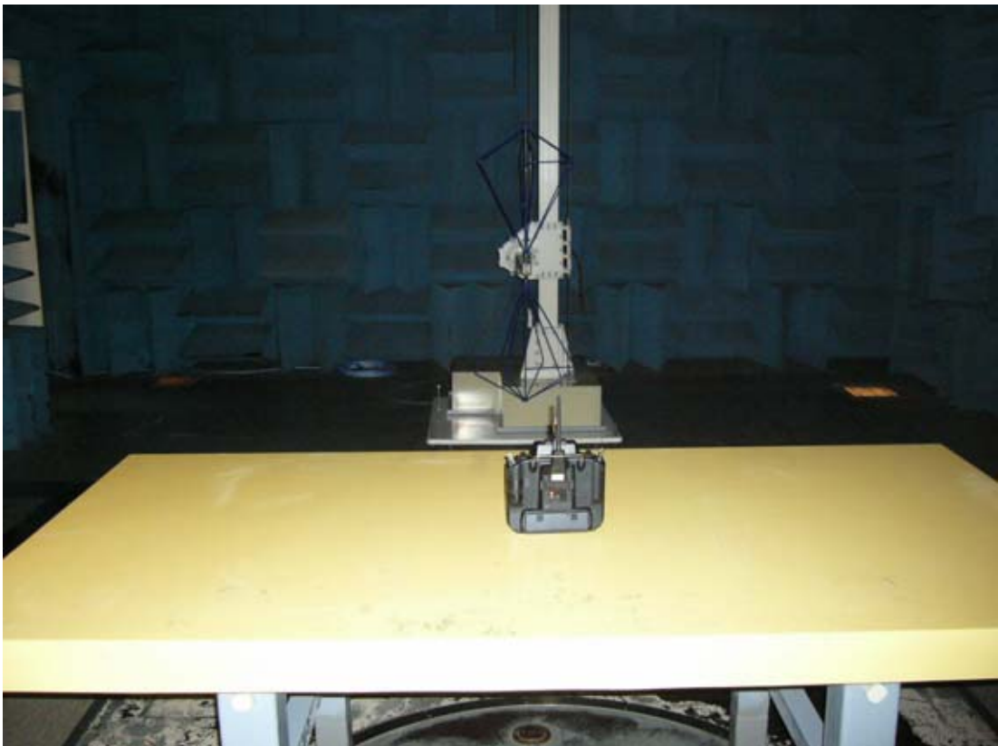
BACK VIEW OF RADIATED MEASUREMENT
