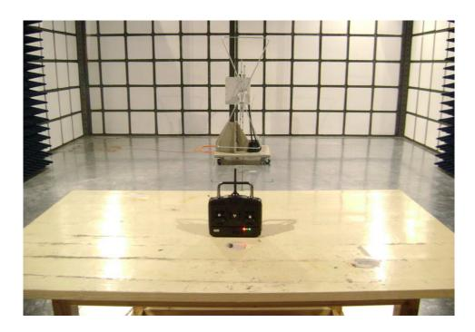
**Radiation Emission Test View For 1GHz-25GHz**
