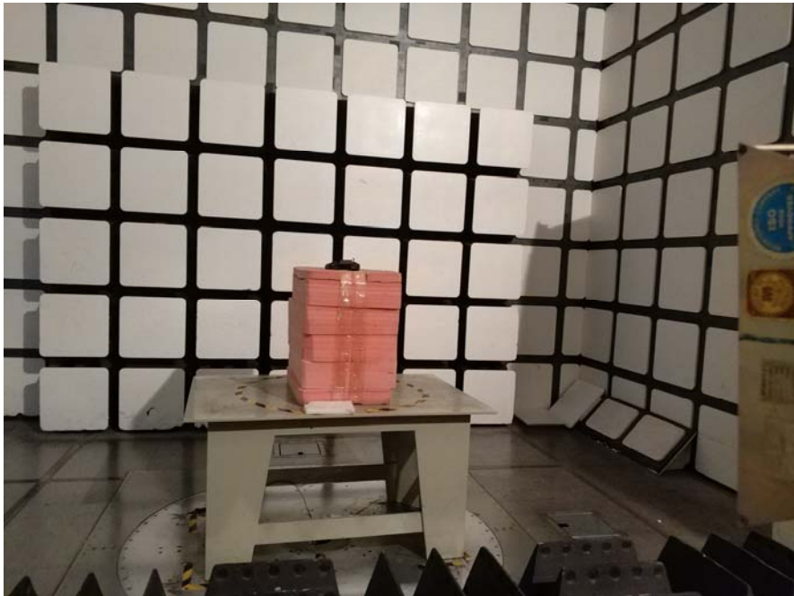
Radiated Emissions View (Above 1 GHz)
