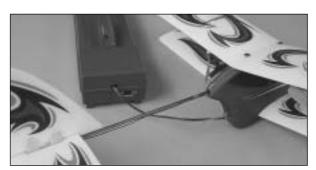
☐ 2. Turn on the charger. Plug the charger cable into the charge socket on the airplane. The charger will plug in only one way.
