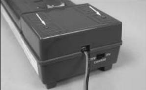
□ 3. Reinstall the battery hatch by replacing the screw and switch on the charger. If the red light is flashing, the charger is ready to be used. If no lights come on, check to make sure that the batteries are installed correctly. If they are, you need to install fresh batteries.
