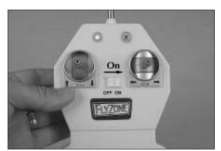
☐ 1. First extend the transmitter antenna. Then switch on the transmitter and make sure the green light is on.
