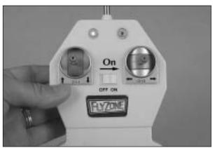
□ 3. Reinstall the battery hatch, switch on the transmitter and check the LEDs on the front of the transmitter. If the green light is on, it is safe to fly. If not, you need to install fresh batteries. Also check to make sure that the batteries are installed correctly.
