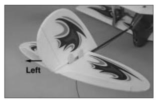
If your airplane turns to the right (E) during glide tests, bend the rudder to the left.
