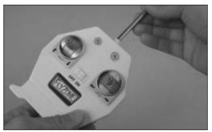
☐ 1. Place the transmitter antenna into the top of the transmitter case as shown above. Tighten it down "clockwise" until it has a snug fit. Do not overtighten the antenna.
