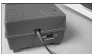
□ 3. Switch on the charger to begin charging. The red LED will flash as long as the battery is charging. Once the battery is charged, the red LED will turn off and the green LED will turn solid. Be aware that during the charging, the green LED will turn on momentarily. Charging should take 5 to 10 minutes.
