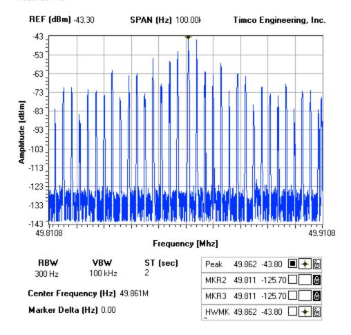
METHOD OF MEASUREMENT: A small sample of the transmitter output was fed into the spectrum analyzer and the attached plot was taken. The vertical scale is set to 10 dB per division. The horizontal scale is set to 5 kHz per division.
