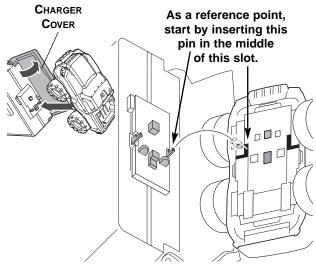
**②** Open the cover on the right side of the transmitter. Position the model parallel to the transmitter with the headlights pointing up. Use the illustrations above to align the model with the pins on the transmitter and snap it into place.
