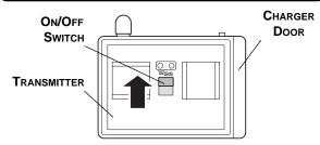
• Set the transmitter switch to ON.
