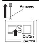
• Gently pull up the antenna by hand. **Never** attempt to extend the antenna by turning or pushing the dial on the back of the transmitter.
