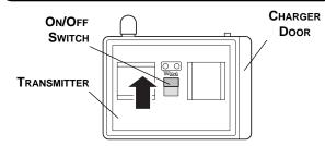
Set the transmitter switch to ON.
