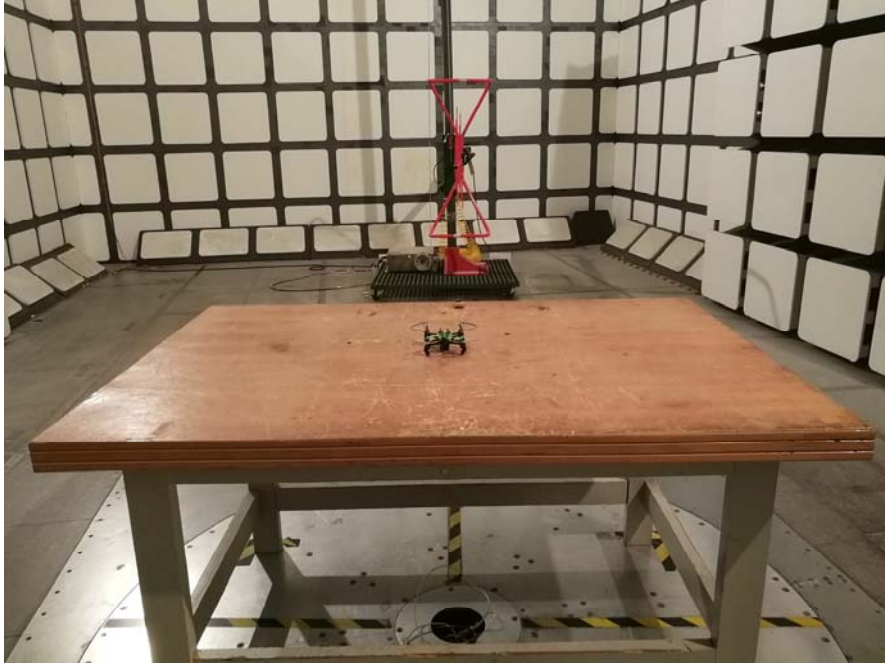
Radiated Emissions View (Below 1 GHz)
