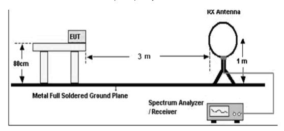
(B) Radiated Emission Test-Up Frequency 30MHz~1GHz
