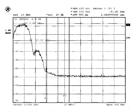
Observation: All emissions in the 100kHz band edge are all lower than carrier by more than 20dB.
