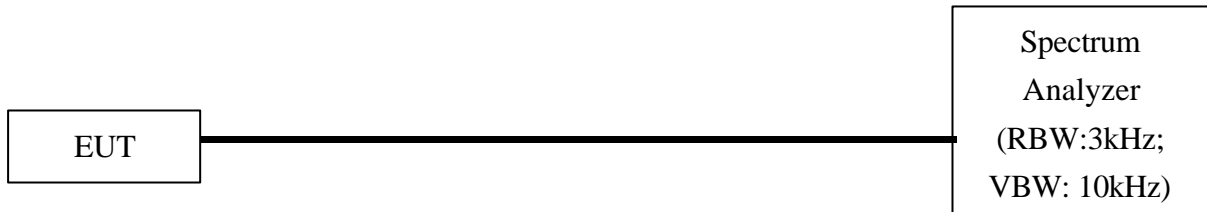
Test Configuration of Power Spectral Density
