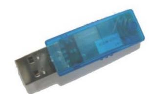
Integrated Antenna Peak Gain @ 2.45GHz: 0.5dBi Coverage 10m ~20m (Varies depending on use environment)
