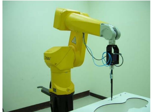
Fig. 5.2 Probe setup on robot
