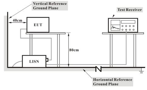
Note: 1. Support units were connected to second LISN. 2. Both of LISNs (AMN) are 80 cm from EUT and at least 80 cm from other units and other metal planes support units.
