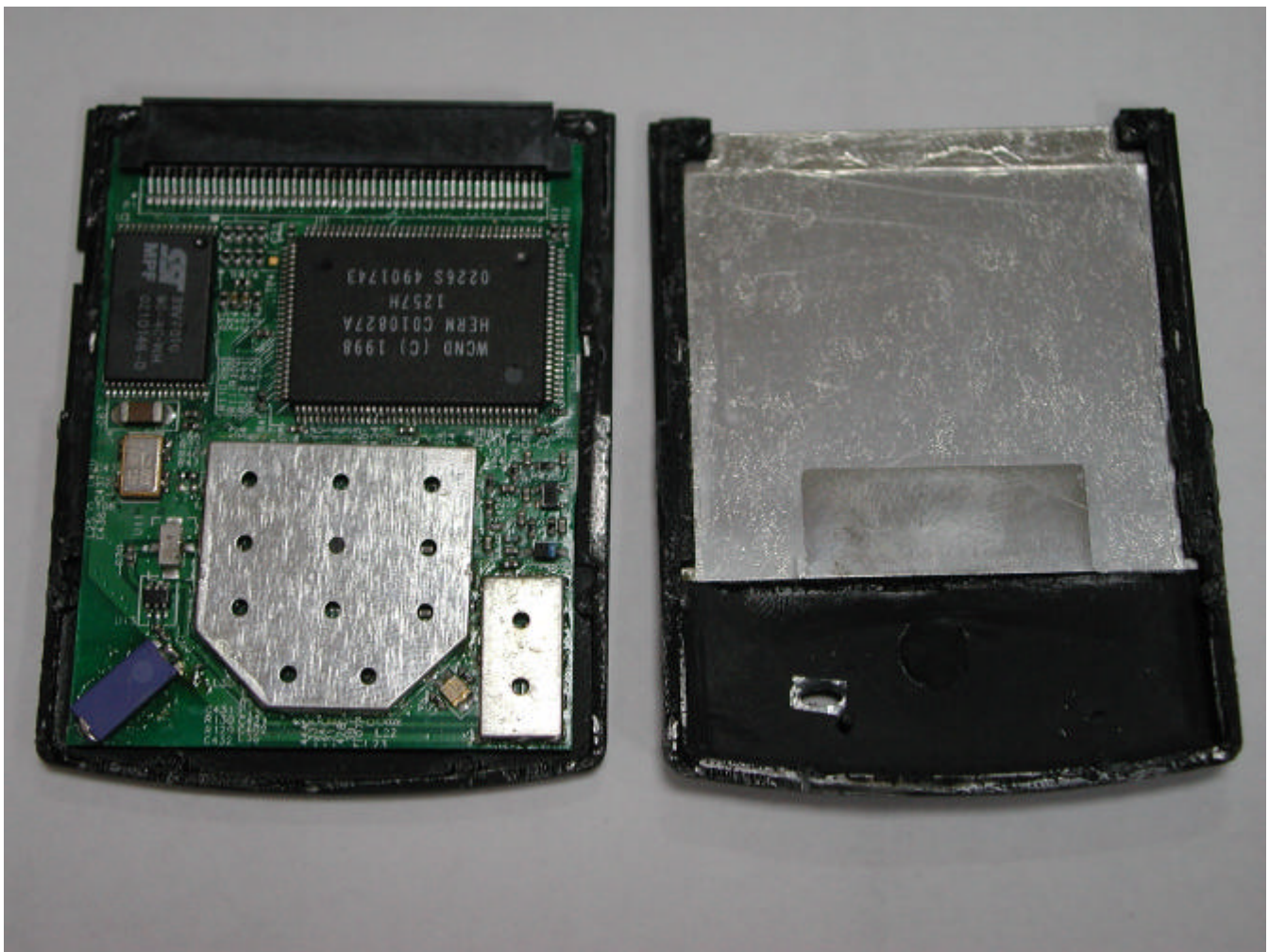
Internal Photo of USI 802.11b CompactFlash Card
