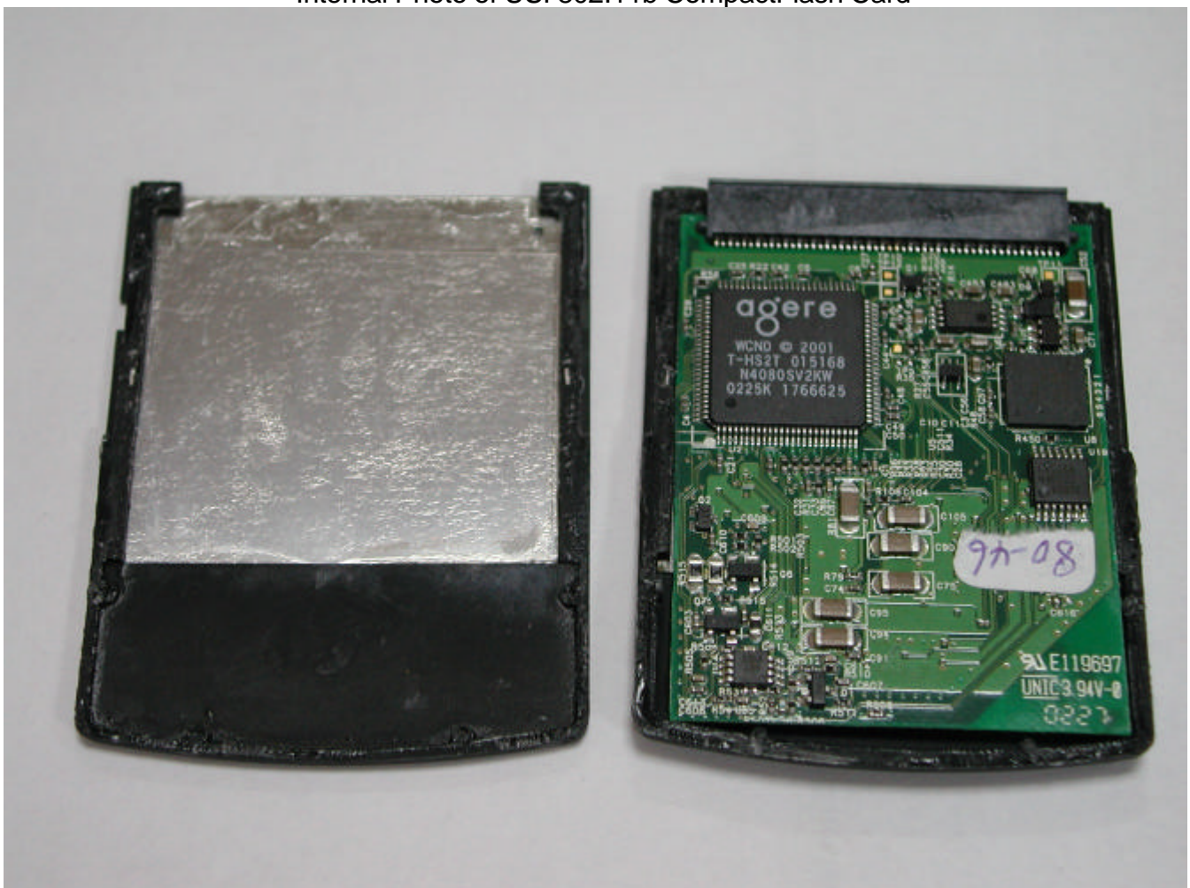
Internal Photo of USI 802.11b CompactFlash Card
